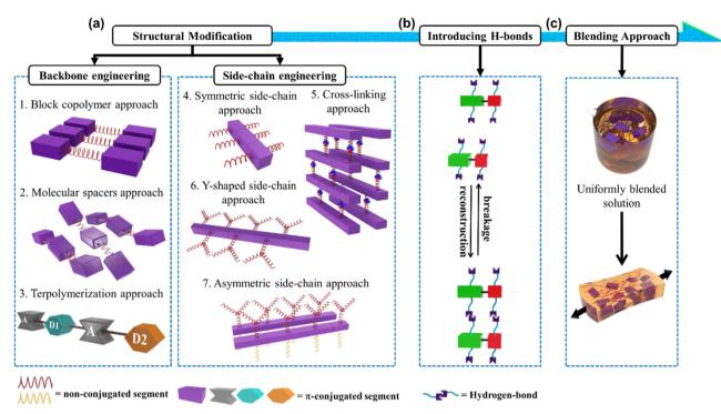
Fig. 1 Illustration of designing novel semiconducting materials to promote mechanical and electrical properties through: (a) structural engineering, which consists of two main strategies, and further divided into seven approaches; (b) functionalizing the side-chain using hydrogen bonding units; and (c) simple blending process of  $\pi$ -conjugated polymer with elastomer matrix, generating autonomous self-healing ability.
