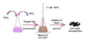
Fig. 3 Steps to synthesize IONPs through the co-precipitation method Fe<sup>2+</sup> and Fe<sup>3+</sup> are added in a 2:1 molar ratio in an oxygen-free environment and heated to 80-85 °C followed by the addition of base. The precipitated particles are then centrifuged or magnetically separated.
