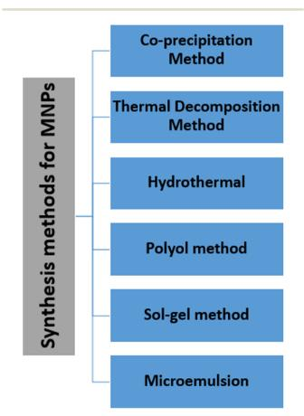
Fig. 2 Various synthetic methods for nanoparticle synthesis.
