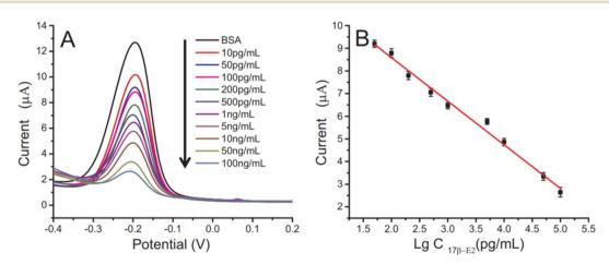
Fig. 12 (A) Differential pulse voltammetry of different concentrations of 17β-E2. (B) Microfluidic paper-based immunodevice calibration curve towards  $17\beta$ -E2. Reproduced from Wang et al. (2018).  $^{131}$
