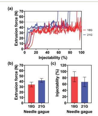
Fig. 5 (a) Extrusion force curves, (b) average extrusion force, and (c) injectability (ratio of injected volume/total volume with extraction force of 50 N) through different needle gauges. Injection medium: sodium alginate with a concentration of 2.5% w/v; Au NP concentration:  $0.5 \text{ g mL}^{-1}$ .
