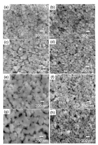
Fig. 10 Scanning electron microscopy (SEM) images of the surface of the sintered copper nanoparticles after sintering at various temperatures. (a,c,e,g) Sintered under  $3\%H_2-N_2$  mixed gas flow, (b,d,f,h) sintered under nitrogen gas flow. Sintering for 1 h at (a and b) 150 °C, (c and d) 180 °C, (e and f) 200 °C, and (g and h) 250 °C.
