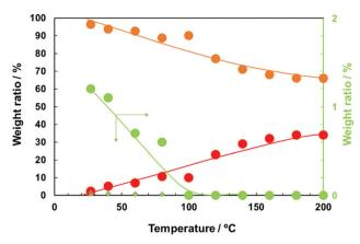
Fig. 6 The weight ratios of Cu (orange left y-axis), Cu<sub>2</sub>O (red left y-axis), and Cu<sub>64</sub>O (small green diamonds: left y-axis, green circle: right y-axis) phases in 1-hexanoic acid-stabilised copper nanoparticles. The weight ratios were calculated from the XRD patterns obtained at high temperatures (Fig. 5) using reference intensity ratio (RIR) calculation.
