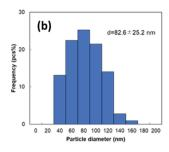
Fig. 1 (a) Transmission electron microscopy (TEM) image and (b) size distribution of 1-hexanoic-acid-stabilised copper nanoparticles prepared by hydrazine reduction of CuO micro particles
