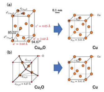
Fig. 13 Schematic illustration of crystalline structural changes during sintering. (a) Cu $_{64}$ O to Cu and (b) Cu $_{2}$ O to Cu.
