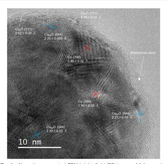
Fig. 4 Aberration-corrected TEM bright-field (BF) image of 1-hexanoicacid-stabilised copper nanoparticles after milling with small zirconia beads (30  $\mu$ m). (ref. Cu(200) 1.808 Å, Cu<sub>64</sub>O(044) 2.215 Å, Cu<sub>2</sub>O(111) 2.465 Å).
