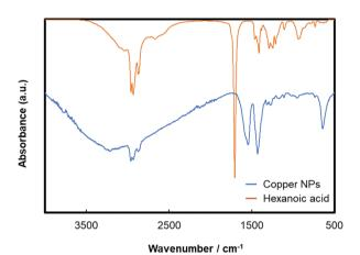
Fig. 2 FT-IR spectra of 1-hexanoic acid (orange) and 1-hexanoic acidstabilised copper nanoparticles (blue) prepared by hydrazine reduction of CuO micro particles. Attribution of the peaks of 1-hexanoic acid: 2976 cm $^{-1}$ , O-H stretch; 1703 cm $^{-1}$ , C=O stretch; 1414 cm $^{-1}$ , O-H bend; 1282 cm<sup>-1</sup> C-O stretch; and 933 cm<sup>-1</sup> O-H bend.
