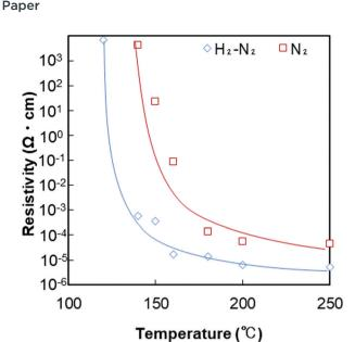
Fig. 8 Relationship between the resistivity of the copper layer film after sintering and the sintering temperature. Red: Sintered under nitrogen gas flow. Blue: Sintered under 3%H<sub>2</sub>-N<sub>2</sub> gas flow.
