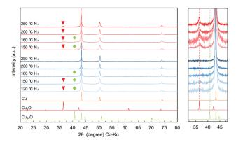
Fig. 9 X-ray diffraction patterns of the copper layers sintered at various temperatures under nitrogen gas flow and  $3\%H_2-N_2$  mixed gas flow. The peak height is normalised to the height of the Cu(111) peak ( $2\theta = 43.3^{\circ}$ ). Red triangle, red broken line:  $Cu_2O(111)$  ( $2\theta = 36.4^\circ$ ). Green diamond, green broken line:  $Cu_{64}O(044)$  (2 $\theta = 40.7^{\circ}$ ).
