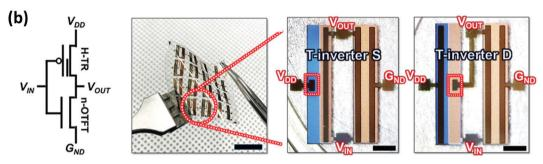
Fig. 14 Performance, illustration, and photographs of flexible MVL circuits produced on plastic substrates. (a) Reprinted with permission from ref. 58 Copyright 2021 The Japan Society of Applied Physics (b) reprinted with permission from ref. 46 Copyright 2021 Wiley-VCH GmbH.
