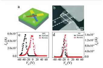
Fig. 6 (a) Illustration and (b) photograph of a cross-bar AAT, where the channels consist of single crystalline OSCs of a quinoidal compound and an anthracene derivative. The transfer curves obtained on the (c) SiO2 and (d) air-gap dielectric layers, indicating that the defect-free air-gap interface is effective in reducing hysteresis. Reprinted with permission from ref. 36 Copyright 2020 The Royal Society of Chemistry
