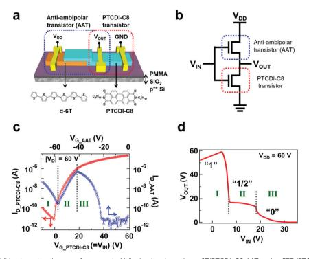
Fig. 8 (a) Illustration and (b) schematic diagram of an organic MVL circuit, where the  $\alpha$ -6T/PTCDI-C8 AAT and n-FET (PTCDI-C8) are connected in series. (c)  $I_D - V_G$  curves for the n-FET (red) and AAT (blue). (d) Voltage transfer curve ( $V_{IN} - V_{OUT}$ ), showing ternary inverter operation. Reprinted with permission from ref. 44 Copyright 2018 American Chemical Society
