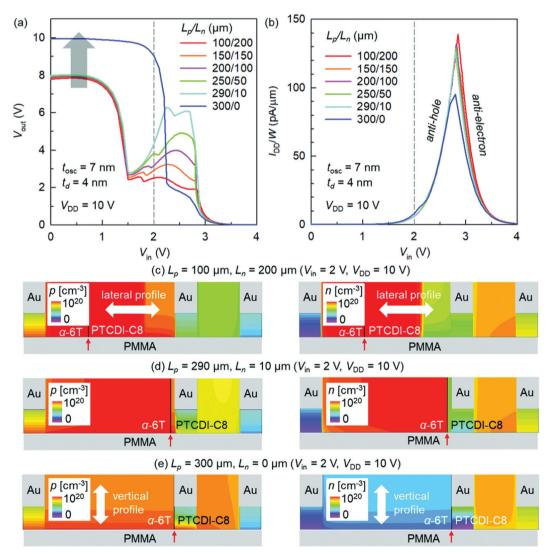
Fig. 11 (a) Voltage transfer curves and (b)  $I_D - V_{IN}$  curves calculated by theoretical simulation, showing clear  $L_D/L_D$  dependence. (c)—(e) Spatial distribution of holes (electrons) on the left (right), depending on  $L_p/L_n$ . Reprinted with permission from ref. 34 Copyright 2021 The Royal Society of Chemistry.
