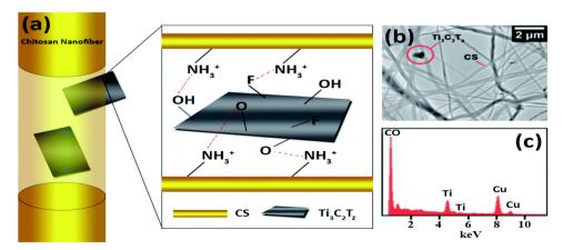
Fig. 8 (a) Schematic representations of the observed orientations of  $Ti_3C_2T_z$  flakes inside chitosan nanofibers. (b) Transmission electron microscopy image of the  $Ti_3C_2T_z/CS$  nano-fibers and (c) elemental examination (presence of copper is attributed to the TEM grid). (Adapted from ref. 143 under Creative Commons License 3.0, Copyright©2018, The Royal Society of Chemistry.)
