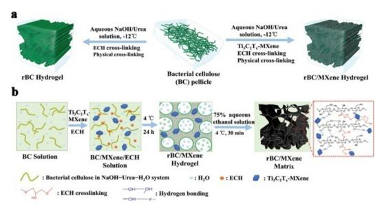
Fig. 5 (a) Schematic outlining the fabrication of rBC-based hydrogels. (b) Diagrammatic representation of the process for developing rBC/MXene composite hydrogels. (Adapted with permission from ref. 141 Copyright © 2021.)
