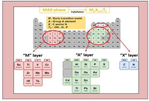
Fig. 1 Composition of the general elements of MXenes and MAX phases, where M is an early transition metal, A is a group A element, X is N and/or C, and  $T_X$  is a surface functional group (adapted from ref. 46 under Creative Commons Attribution 4.0).
