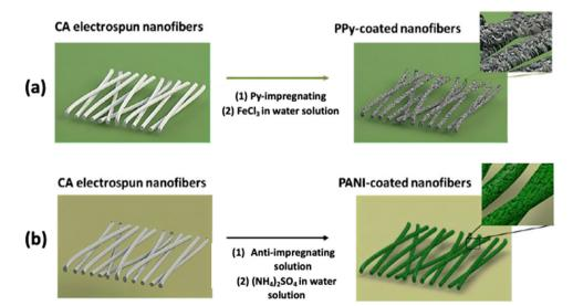
Fig. 5 The procedure followed to prepare CA fibers with (a) PPy and (b) PANI by in situ chemical polymerization. Reproduced from ref. 74 with permission from the Royal Society of Chemistry.
