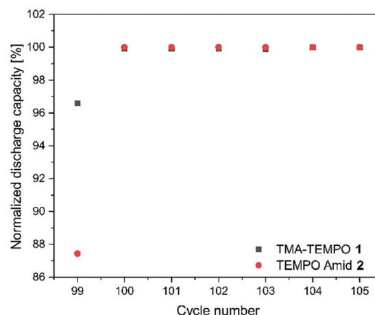
**Fig. 1** Illustration of the discharge capacity of the first seven cycles of the TMA-TEMPO **1** and the amide **2** after the second hold time of 24 h. The capacity was normalized to the highest capacity in the shown interval. The first cycle showed a massively reduced discharge capacity.
