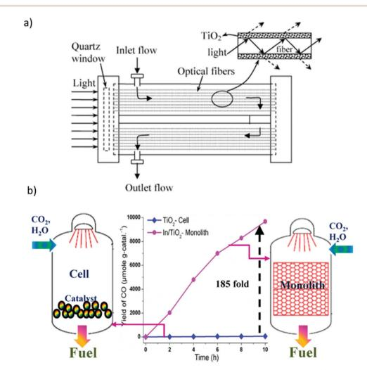
Fig. 11 (a) Schematic diagram of an optical fiber reactor, reproduced with permission from ref. 181, Copyright 2007, Elsevier. (b) Comparison of photocatalytic  $CO_2$  reduction with  $H_2O$  using cell- and monolith-type photoreactors. Reproduced with permission from ref. 170, Copyright 2013, Elsevier.
