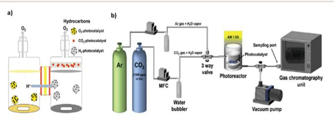
**Fig. 10** Illustration of two setups for photocatalytic CO<sub>2</sub> reduction: (a) twin reactor. Reproduced with permission from ref. 177, Copyright 2018, Elsevier. (b) Continuous-flow reactor. Reproduced with permission from ref. 93, Copyright 2017, Elsevier.
