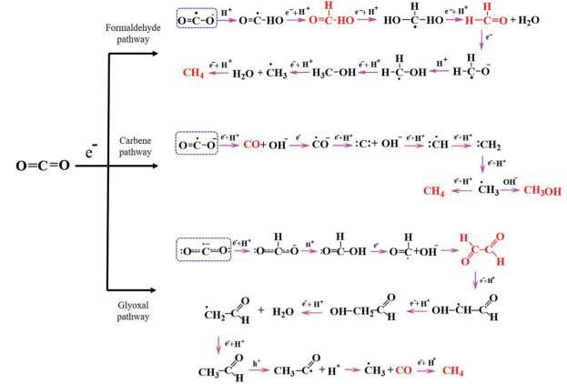
Fig. 5 General pathways for photocatalytic CO<sub>2</sub> reduction: formaldehyde, carbene, and glyoxal. Adapted from ref. 9, Copyright 2020, Royal Society of Chemistry.
