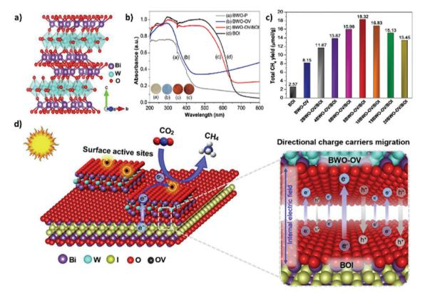
Fig. 15 (a) Crystal structure of oxygen-deficient  $Bi_2WO_6$ , (b) UV-vis absorption spectra of various samples, (c) photocatalytic  $CO_2$  reduction activity of various catalysts toward  $CH_4$  formation, and (d) schematic illustration of the  $CO_2$  reduction mechanism on the  $Bi_2WO_6/BOI$  composite. Reproduced with permission from ref. 262, Copyright 2019, Elsevier.
