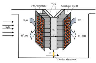
**Fig. 12** Schematic diagram of a monolithic two-sided Cu<sub>2</sub>O/graphene/ TNA photoreduction reaction system. Reproduced with permission from ref. 186, Copyright 2016, Elsevier.
