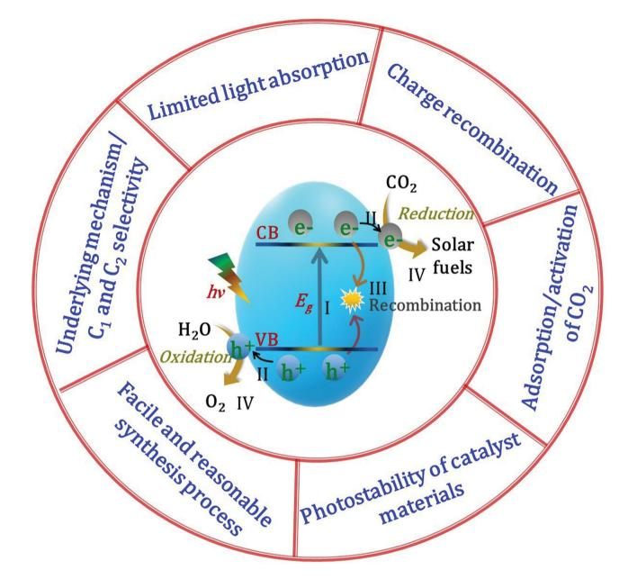
Fig. 2 Schematic illustration and challenges of the photocatalytic CO<sub>2</sub> conversion process.
