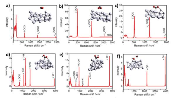
**Fig. 22** (a) Physisorbed  $CO_2$ , (b)  $CO_2^{\delta^-}$  anion with both O atoms facing the  $Ag^{\delta^+}$  surface, (c)  $CO_2^{\delta^-}$  anion binding to the  $Ag^{\delta^+}$  surface *via* C and O atoms, (d) HOCO\* intermediate bound to the Ag surface *via* a C atom, and (f) surface-bound CO\* and OH\* formed from dissociation of a HOCO\* intermediate with both O atoms facing the Ag surface. Reproduced with permission from ref. 396, Copyright 2018, American Chemical Society.
