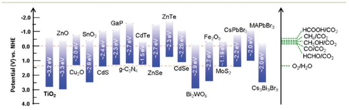
Fig. 3 Band potentials and corresponding bandgap energies of various selected photocatalysts relative to the redox potential involved in CO<sub>2</sub> photoreduction to various products.
