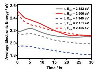
Fig. 11 Time evolution of the average electronic energy value  $\bar{E}$  after optical excitation in the ZnPc aggregates. The solid and dashed lines are results of the  $\alpha$  and  $\beta$  phases, respectively.
