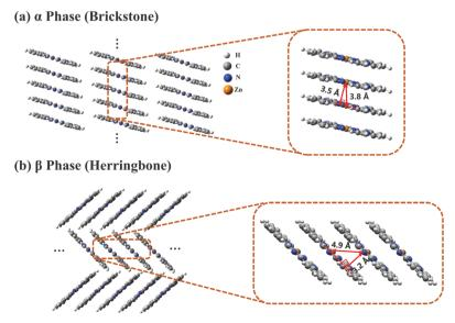
Fig. 1 Crystal stacking structures of (a) α-phase and (b) β-phase ZnPc aggregates. The two magnification boxes present the structures of the ZnPc tetramers extracted from the corresponding aggregates.
