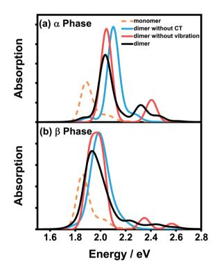
Fig. 4 Vibrationally resolved absorption spectra of the ZnPc dimer with the (a)  $\alpha$ -phase and (b)  $\beta$ -phase configurations in a mixed solvent of N-methylpyrrolidone and chloroform. The corresponding monomer spectrum (orange dashed line) is also shown for comparison. All of the calculated spectra are broadened using the Gaussian line shape function with a full width of 0.1 eV.
