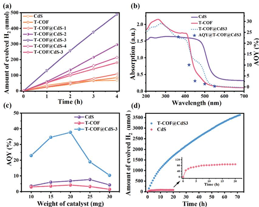
Fig. 5 (a) Time course of H<sub>2</sub> evolution over various catalysts (10 mg). (b) AQY values of T-COF@CdS-3 (10 mg) under different monochromatic light irradiation and UV-visible DRS spectra. (c) AQY values of CdS, T-COF and T-COF@CdS-3 at different photocatalyst weights under 365 nm monochromatic light irradiation. (d) Photocatalytic durability test results of T-COF@CdS-3 and CdS.
