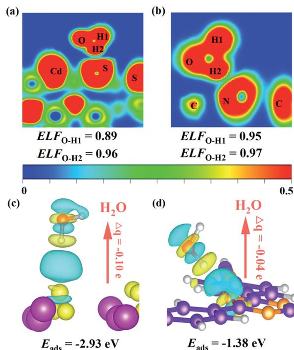
Fig. 6 Electronic local functions (ELFs) of (a) CdS and (b) T-COF after adsorption of  $H_2O$ . The charge density difference of water adsorption on (c) CdS and (d) T-COF.  $E_{ads}$  is the adsorption energy and  $\Delta q$  is the Bader charge.
