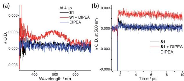
Fig. 2 (a) ns-TA spectra recorded at 4  $\mu$ s after pulse excitation at 355 nm, and (b)  $\Delta$ O.D. intensity at 500 nm for degassed MeCN solutions containing **S1** (0.1 M; black line), **S1** (0.1 M) and DIPEA (0.25 M; red line) or DIPEA (0.25 M; blue line).
