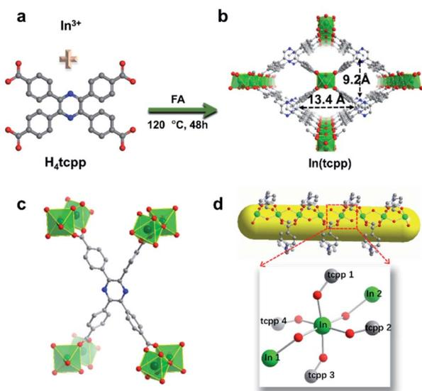
Fig. 1 Representation of the crystal structure of In(tcpp). (a) The organic and inorganic building units of In(tcpp) and reaction conditions. (b) The one-dimensional channel in In(tcpp). (c) The coordination of the tcpp ligand. (d) The 6-coordinated In<sup>3+</sup> ion and 1D In<sup>3+</sup> chain along the *a*-axis. Color code: C grey; N blue; O red; In green; H atoms are omitted.
