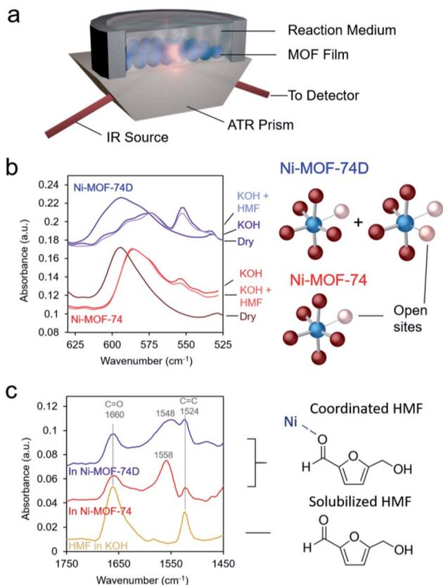
**Fig. 3** An ATR configuration was used to probe the MOF-HMF interactions (a). The low wavenumber spectra reveal that Ni-MOF-74D has more open coordination sites in which OH can adsorb, which is then partially displaced by HMF (b). The HMF-Ni interactions can also be visualized in the high wavenumber region in which a new band arises, stemming from the interaction of the HMF aldehyde group with the Ni centers of the MOFs (c).
