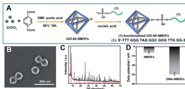
Fig. 1 (A) Synthesis of the nucleic acid (1)-functionalized UiO-66 NMOFs. (B) SEM image of the (1)-modified UiO-66 NMOFs. (C) XRD pattern of the UiO-66 NMOFs (black), and simulated XRD pattern of the UiO-66 NMOFs (red). (D) Zeta-potentials corresponding to the bare UiO-66-NMOFs and the nucleic acid (1)-functionalized UiO-66 NMOFs. Error bars derived from  $N = 3$  experiments.
