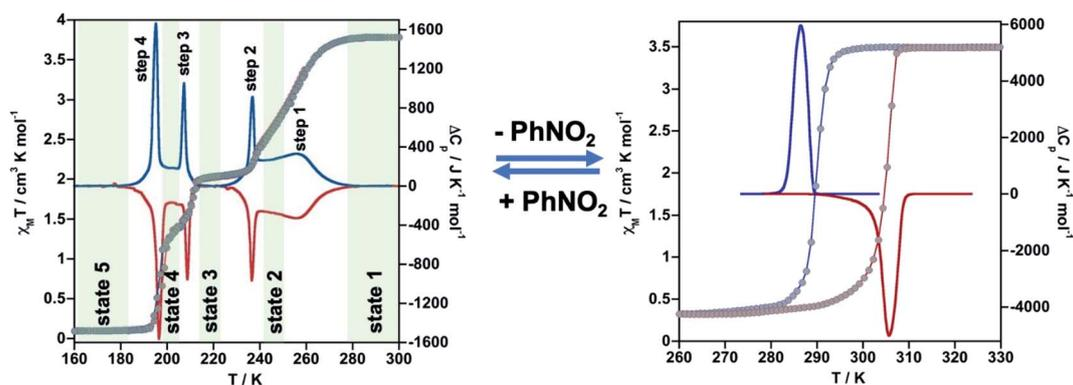
Fig. 1 Thermal dependence of magnetic (grey circles) and calorimetric properties of  $1 \cdot \text{PhNO}_2$  (left) and  $1$  (right). Blue and red curves correspond to the cooling and heating modes in  $\Delta C_p$ .
