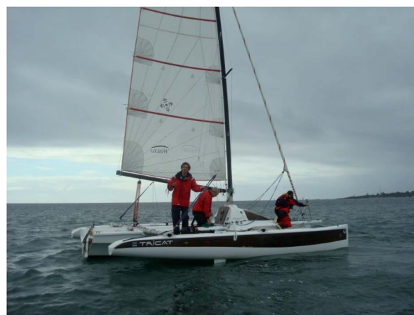
Fig. 3 Gwalaz, flax fibre reinforced trimaran.
