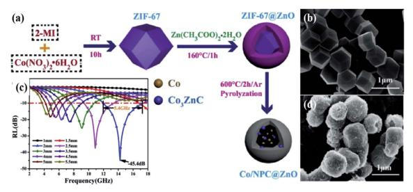
Fig. 6 The scheme for the synthesis of Co/NPC@ZnO/rGO (a), SEM images of ZIF-67 (b) and Co/NPC@ZnO/rGO (d), and the RL of Co/NPC@ZnO/rGO (c). This figure has been adapted from ref. 97 with permission from Journal of alloys and compound, Copyright 2020.
