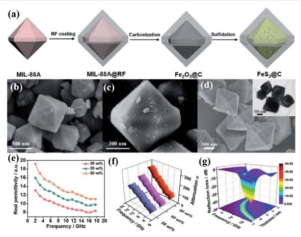
Fig. 9 The schematic formation process of FeS<sub>2</sub>/C composites (a), SEM images of Fe-MOF (b), Fe<sub>3</sub>O<sub>4</sub>/C (c), SEM and TEM images of FeS<sub>2</sub>/C (d), the real permittivity (e), attenuation constant (f) and the RL of  $FeS_2/C$  composites (g). This figure has been reproduced from ref. 16 with permission from Nano Letters, Copyright 2020.
