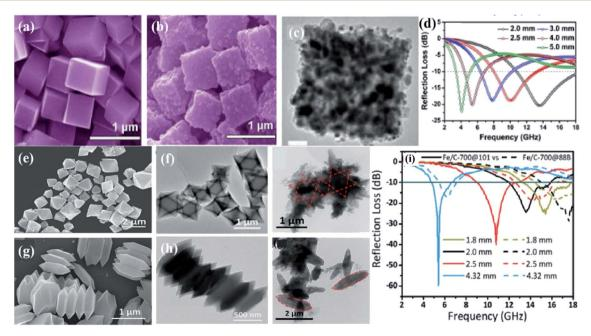
Fig. 4 SEM and TEM images of PB (a), Fe/C-PB (b and c), MIL-101-Fe (e), Fe/Fe<sub>3</sub>C/C-800@101 (f), MIL-88B-Fe (g), and Fe/Fe<sub>3</sub>C/C-800@88B (h), respectively. RL of Fe/C-PB (d), Fe/C-700@101 and Fe/C-700@88B (i), respectively. This figure has been reproduced from ref. 18 and 83 with permission from Advanced Materials Interfaces, Copyright 2020 and Journal of Materials Chemistry A, Copyright 2015.
