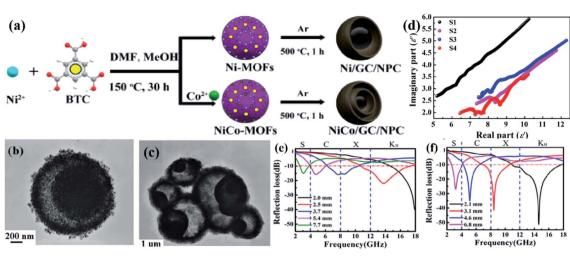
Fig. 8 The schematic formation process of the NiCo/GC/NPC composites (a), TEM images of S1 (b), S4 (c), the Cole-Cole semicircles of S1-S4 (d), the RL with various thicknesses for S1 (e), S4 (f) (S1 represents Ni/GC/NPC, and the content of Co increases from S1 to S4). This figure has been reproduced from ref. 71 with permission from Applied Surface Science, Copyright 2020.
