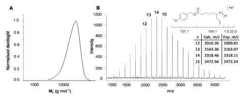
Fig. 2 (a) Size exclusion chromatogram of the molecular weight distribution of  $A_{\epsilon}PCL$  using 4-methoxybenzyl alcohol as initiator ( $[M_0]/[I_0] = 50$ ). Molecular weight was determined against poly(styrene) standards using CHCl<sub>3</sub> (0.5% NEt<sub>3</sub>) as eluent. (b) MALDI ToF-MS of  $A_{\epsilon}PCL$  initiated by 4-methoxybenzyl alcohol.
