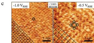
Fig. 5 (a) Schematic of *in situ* EC-STM setup. Copyright 2018, John Wiley and Sons; (b) schematic of *in situ* EC-AFM; (c) morphology of Cu surface at different potentials characterized by *in situ* AFM. Copyright 2020, John Wiley and Sons. All panels reproduced with permission. 139,143
