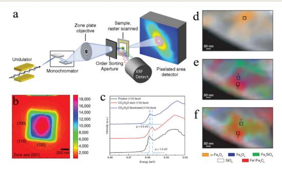
Fig. 7 (a) STXM and SFXM setup; Copyright 2014, National Academy of Sciences; (b) SFXM image of a Cu<sub>2</sub>O nanoparticle; (c) scanning X-ray nanospectroscopy of the (110) facet; Copyright 2019, Springer Nature; (d) to (f) chemical contour images of the catalyst under different treatments; Copyright 2008, Springer Nature. All panels reproduced with permission.  $^{148,156,160}$
