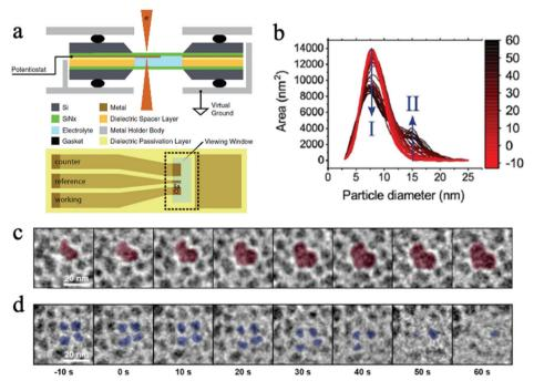
Fig. 6 (a) The schematic of a micro electrochemical cell for in situ TEM. Copyright 2017, IOP Publishing, Inc.; (b) the change in primary (l) and secondary (II) particle sizes as experiment progresses; (c) the growth of secondary particles, and (d) the shrinkage of primary particles. Copyright 2020, John Wiley and Sons. All panels reproduced with permission. 152,154
