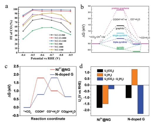
Fig. 2 (a) FE of catalysts with different surface areas. Copyright 2021, Springer Nature; (b) free energy diagram of  $CO_2$  ECR to CO on different NG surfaces. Copyright 2016, American Chemical Society; (c) free energy diagrams and (d) the calculated limiting potentials for  $CO_2$ RR and HER on composite and pristine graphene surfaces. Copyright 2018, John Wiley and Sons. All panels reproduced with permission.  $^{23,92,96}$
