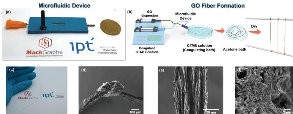
**Fig. 1** (a) Photograph of the 3D hydrodynamic flow focusing microfluidic (3DHFFM) device fabricated to obtain the GO microfibers. (b) Illustration of GO microfiber formation. (c) Photograph of the GO microfiber. SEM images of the GO microfibers (d) with an overhand knot, and (e) of the surface and (f) cross section. The GO microfibers are flexible, and their surfaces are not smooth, with many dentate-bends.
