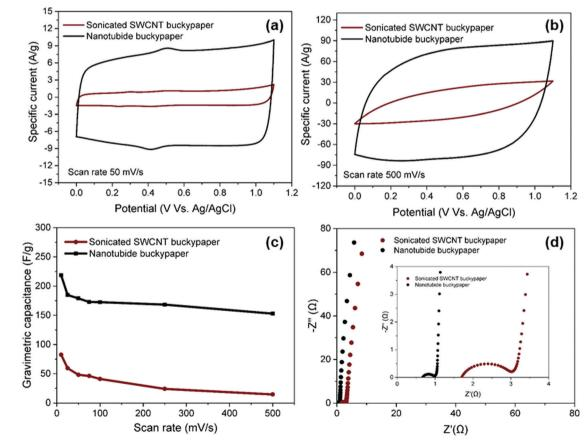
Fig. 3 Half-cell electrochemical performance, in 1 M  $H_2SO_4$ , comparing optimised nanotubide buckypaper to a conventionally processed control: (a) CV curves at 50 mV s<sup>-1</sup>, (b) CV curves at 500 mV s<sup>-1</sup>, (c) gravimetric capacitance as a function of scan rate normalised by mass of active electrode and (d) Nyquist plots.
