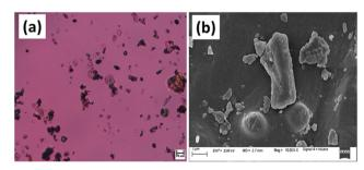
Fig. 1 (a) A POM image and (b) an FESEM image of bamboo-root flour particles
