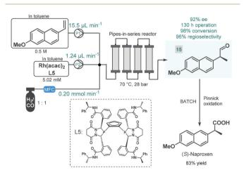
Scheme 6 Continuous flow enantioselective synthesis of a chiral naproxen precursor. <sup>62</sup>
