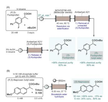
Scheme 16 Continuous flow biocatalytic synthesis of chiral propionic acid-derived APIs. <sup>101,108</sup> (BS2M = esterase from *Bacillus subtilis*).
