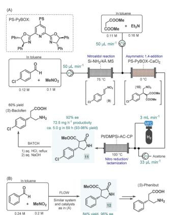
Scheme 4 Multistep continuous flow asymmetric synthesis of chiral baclofen and phenibut precursors. 55,57
