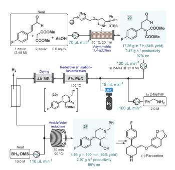
**Scheme 11** Continuous flow enantioselective synthesis of the key phenylpiperidine intermediate of (–)-paroxetine. <sup>86</sup>
