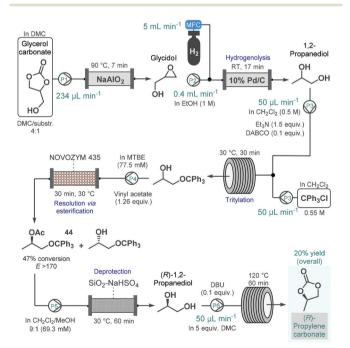
**Scheme 19** Step-wise continuous flow synthesis of (R)-propylene carbonate using a chemoenzymatic resolution as key step to introduce asymmetry. 114 (DABCO = 1,4-diazabicyclo[2.2.2]octane, DBU = 1,8-diazabicyclo[5.4.0]undec-7-ene).
