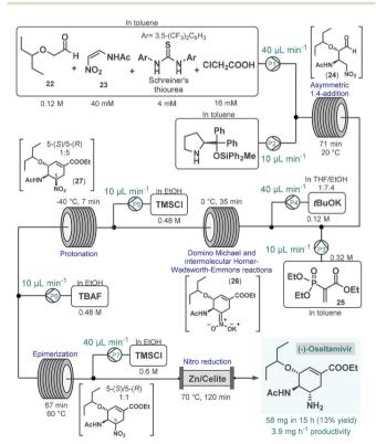
Scheme 10 Five-step telescoped continuous flow asymmetric organocatalytic synthesis of (–)-oseltamivir.<sup>82</sup>
