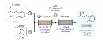
Scheme 17 Synthesis of mexiletine via continuous flow biocatalytic asymmetric amination. (TA =  $\omega$ -transaminase from Arthrobacter).
