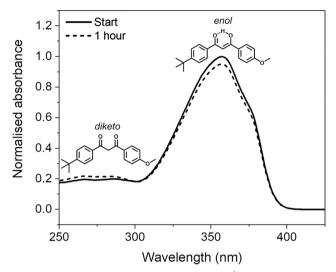
Fig. 1 Normalised UV-visible spectra of 5  $\mu$ g mL<sup>-1</sup> ( $\sim$ 16  $\mu$ M) solution of avobenzone in ethanol taken before and after one hour of irradiation (solid and dotted lines, respectively), using a xenon lamp at solar irradiance (~1000 W m<sup>-2</sup>). Inset are the molecular structures of the chelated enol and diketo tautomers of avobenzone that give rise to the spectral peaks at  $\sim$  350 nm and  $\sim$  270 nm, respectively
