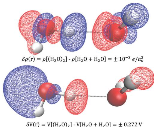
Fig. 11 Deformation densities  $\delta\rho(\mathbf{r})$  (top) and electric potentials  $\delta V(\mathbf{r})$  (bottom) when two water molecules are brought together:  $\text{H}_2\text{O} + \text{H}_2\text{O} \rightarrow (\text{H}_2\text{O})_2$ . The blue and red isosurfaces denote increases (+) and decreases (−), respectively. Small changes in electron density yield large changes in electric potentials. QM level: B3LYP/6-31+G\*.
