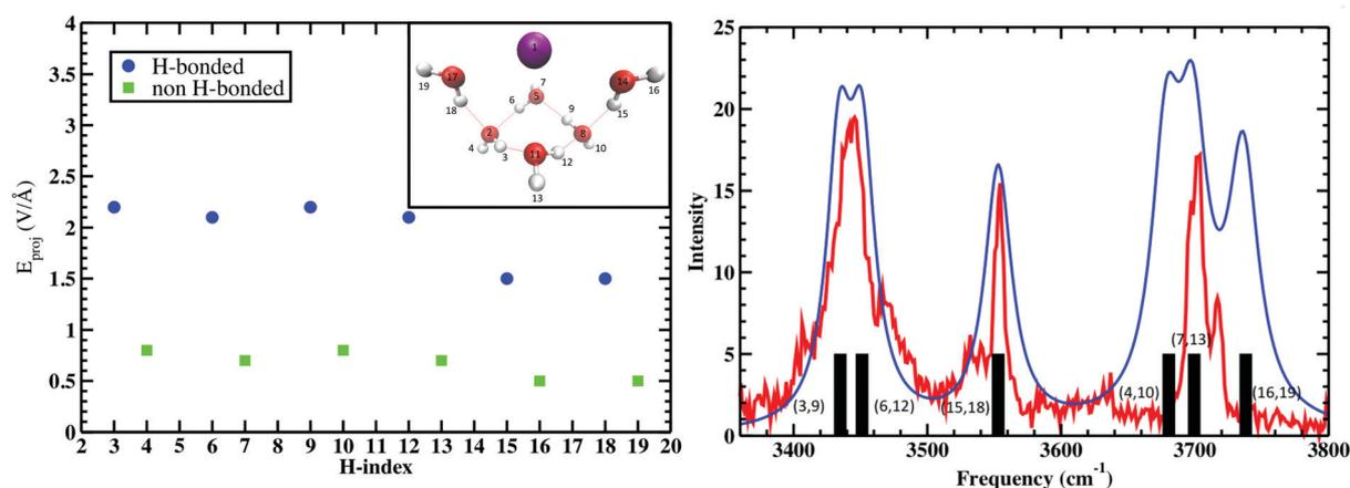
Fig. 4 (Left) Projected QM  $E$  fields (left) on the H atoms in Cs<sup>+</sup>(H<sub>2</sub>O)<sub>6</sub> where the blue and green symbols denote those OH groups that are H-bonded and free, respectively (the H-indices correspond to those in the inset). (Right) Comparison of the measured vibrational spectra (red) and that from the projected QM fields (black bars) and Lorentzian fits to QM fields (blue). See Wolke *et al.*<sup>56</sup> for more details. QM level: MP2/aug-cc-pVDZ.
