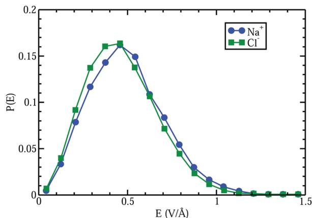
Fig. 10 Comparison of electric field distributions at the locations of the Na<sup>+</sup> and Cl<sup>-</sup> ions from CL simulations of a 6.7 M aqueous NaCl electrolyte.
