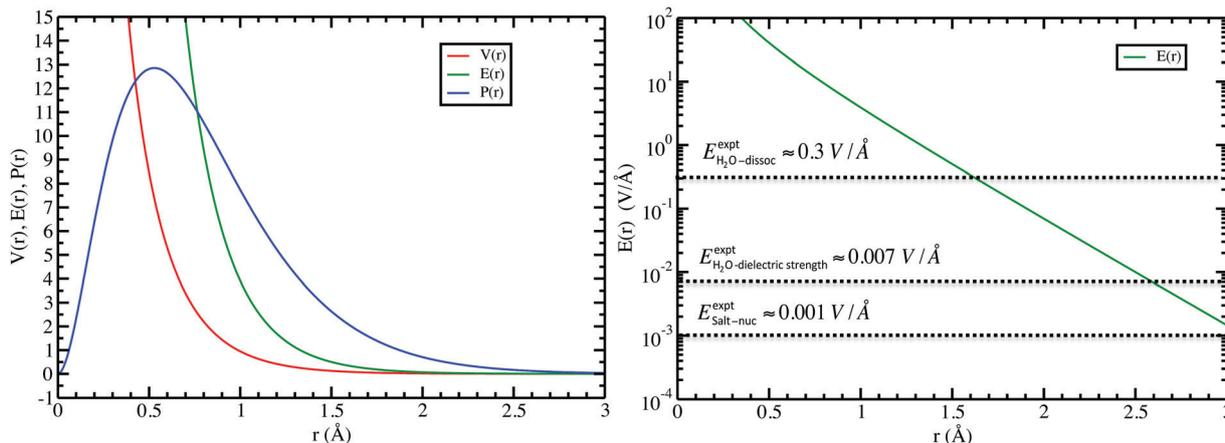
Fig. 1 Quantum electric potential  $V(r)$ , field  $E(r)$ , and scaled radial probability  $4\pi P(r)$  for the “neutral” hydrogen atom (left), and (right) a few reference field strengths compared to that from hydrogen (note vertical log-scale): for  $\text{H}_2\text{O}$  dissociation,  $\text{H}_2\text{O}$  dielectric strength, and that required to induce KCl salt nucleation.
