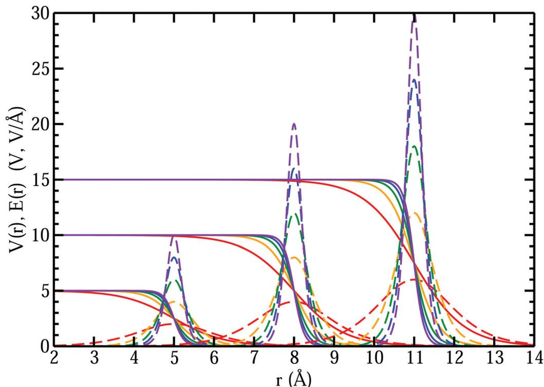
Fig. 13 Comparison of interfacial electric potentials (solid) and corresponding fields (dashed) for different MIPs ( $V_o = 5, 10, 15$  V), interface locations ( $R = 5, 8, 11$  Å), and width parameters ( $k = 0.8$  (red), 1.6 (orange), 2.4 (green), 3.2 (blue), 4.0 (purple) Å<sup>-1</sup>).
