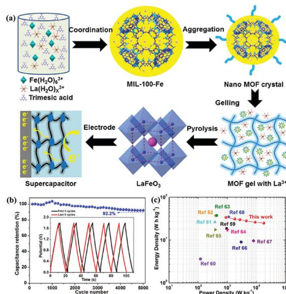
Fig. 5 (a) Schematic illustrations showing the synthesis of perovskite LaFeO<sub>3</sub>. (b) Cycling stability versus cycle number graph, inset: the first and last five GCD cycles. (c) Ragone plots (energy density vs. power density) of this work and other devices. Reproduced from ref. 61 with permission from Elsevier B.V., copyright 2020.
