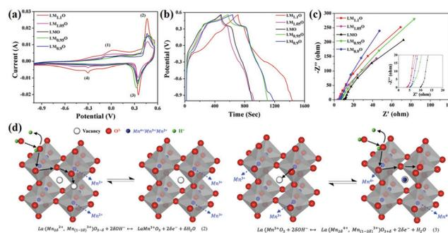
**Fig. 6** (a) Cyclic performance of the LM<sub>1±x</sub>O<sub>3</sub> samples at a scan rate of 0.01 V s<sup>-1</sup>. (b) Charge–discharge curves in a potential window of –1 to 0.56 V at 1 A g<sup>-1</sup>. (c) EIS of the LM<sub>1±x</sub>O<sub>3</sub> samples with the inset of enlarged R<sub>s</sub> at high frequencies. (d) Charge storage mechanism in LM<sub>1±x</sub>O<sub>3</sub> perovskite oxide materials. Reproduced from ref. 91 with permission from Elsevier B.V., copyright 2017.
