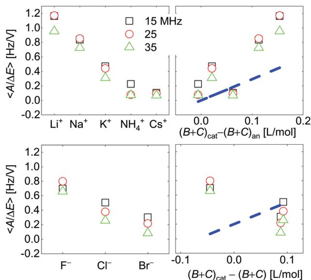
**Fig. 7** Voltage-normalized amplitudes for a set of cations (top) and a set of anions (bottom). The right-hand side shows the data plotted versus  $\sum(B_i + C_i)/z_i$ . The dashed blue line indicates the slope as predicted from eqn (8) and (9). Ions were ordered according to ion radius on the left-hand side. Fractional errors of the mean: cations: 0.6%; anions: 1.8%.
