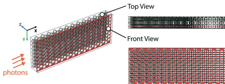
Fig. 3 Geometry of the modeled control volume (2.5 mm × 0.98 mm × 0.38 mm) of the 5 mm ID glass bead reactor, which contains three layers of close-packed glass beads (diameter = 100 μm). In each layer, there are 26 columns × 8 rows of glass beads (front view).
