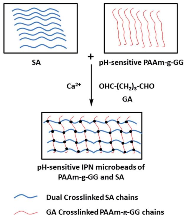
Fig. 4 Formation mechanism of sodium alginate-based IPN gel microspheres with double cross-linking of  $\text{Ca}^{2+}$  + GA. This figure has been adapted from ref. 53 with permission from Elsevier B.V., copyright © 2015.
