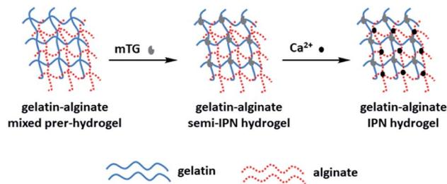
Fig. 5 Formation mechanism of sodium alginate-based IPN hydrogel with double cross-linked of Enzyme and ion. This figure has been adapted from ref. 54 with permission from WILEY-VCH Verlag GmbH & Co. KGaA, Weinheim, copyright © 2014.
