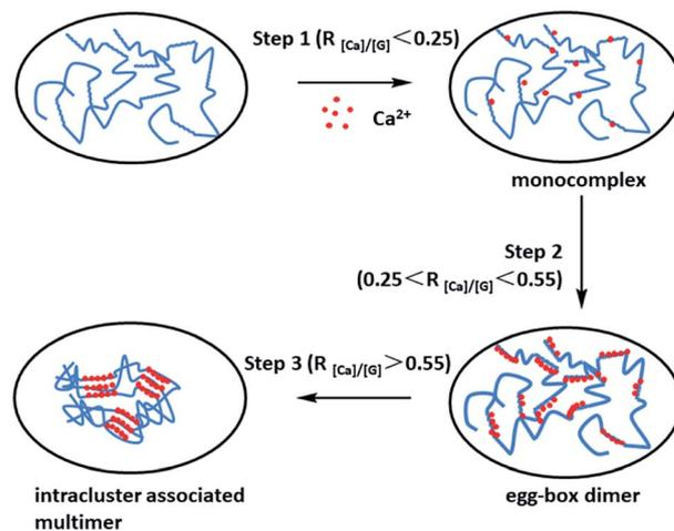
Fig. 1 Schematic drawing of the multiple-step binding of  $\text{Ca}^{2+}$  to alginate with a considerable chain length. The zigzag lines, smooth lines, and dots stand for G-block, M-block, and  $\text{Ca}^{2+}$ , respectively.  $R_{[\text{Ca}]/[\text{G}]}$  is the feeding ratio of added  $\text{Ca}^{2+}$  to unit G residue. This figure has been adapted from ref. 50 with permission from American Chemical Society, Copyright © 2007.
