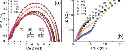
Fig. 13 Cole-Cole plots of the 0-20% cobalt doped ZnO/CuO heterojunction solar cells. Insets indicate the equivalent circuit model, (b) Magnified view of Cole-Cole plots in the high-frequency region.
