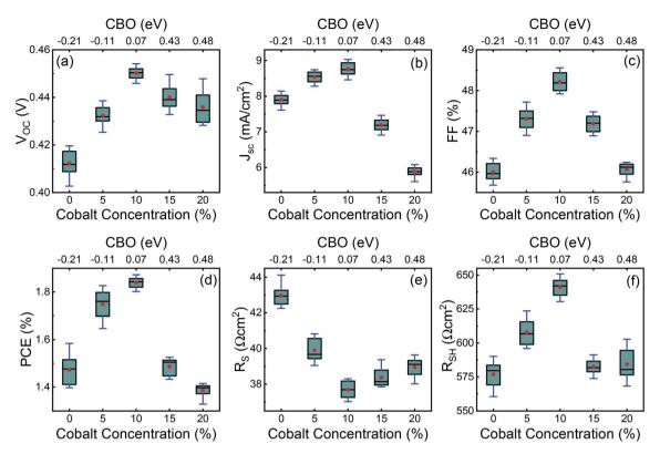
Fig. 10 Statistics of device performance using various cobalt doped ZnO window layer (0-20%). (a) Open circuit voltage  $(V_{OC})$ , (b) short circuit current density  $(J_{SC})$ , (c) fill factor (FF), (d) power conversion efficiency (PCE), (e) series resistance  $(R_S)$ , and (f) shunt resistance  $(R_{SH})$ . The solid red circle represents the average values, and the horizontal lines in the box denote the 25th, 50th, and 75th percentile values.
