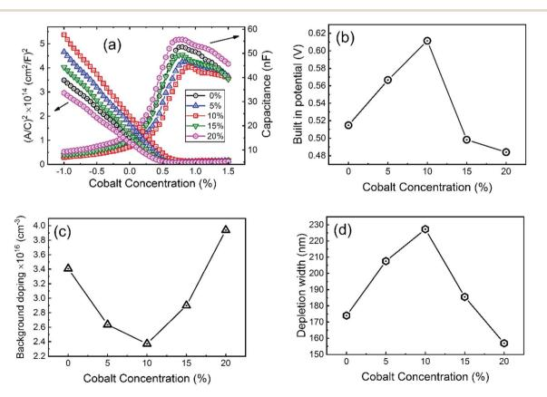
Fig. 14 (a) Capacitance–voltage (C-V) and Mott–Schottky plots of the 0–20% cobalt doped ZnO/CuO heterojunction solar cells. Variation in (b) built-in potential, (c) background doping concentration, and (d) depletion width as a function of cobalt concentration.
