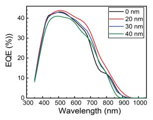
Fig. 16 EQE spectra of ZnO/CuO/MoO<sub>3</sub> heterojunction solar cells.
