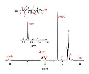
Fig. 3 <sup>1</sup>H NMR spectrum of poly(L-alanine) with an alkyne moiety at the N-terminus synthesized via papain-catalyzed polymerization at the Ala-OEt/2 feed ratio of 1/0.2. Asterisk shows spinning side bands of solvent peak.
