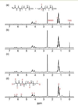
Fig. 1 <sup>1</sup>H NMR spectra of poly(L-alanine)s with an acrylamide moiety at the N-terminus synthesized via papain-catalyzed polymerization at different Ala-OEt/1 feed ratios: (a) Ala-OEt/1 = 1/0.1, (b) Ala-OEt/1 = 1/0.3, (c) Ala-OEt/1 = 1/0.5, and (d) Ala-OEt/1 = 1/1.
