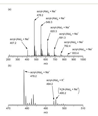
Fig. 2 (a) MALDI-TOF MS spectrum of poly(L-alanine)s with an acrylamide moiety at the N-terminus synthesized via papain-catalyzed polymerization at an Ala-OEt/1 feed ratio of 1/1 and (b) the expanded spectrum from 470 to 510 m/z.
