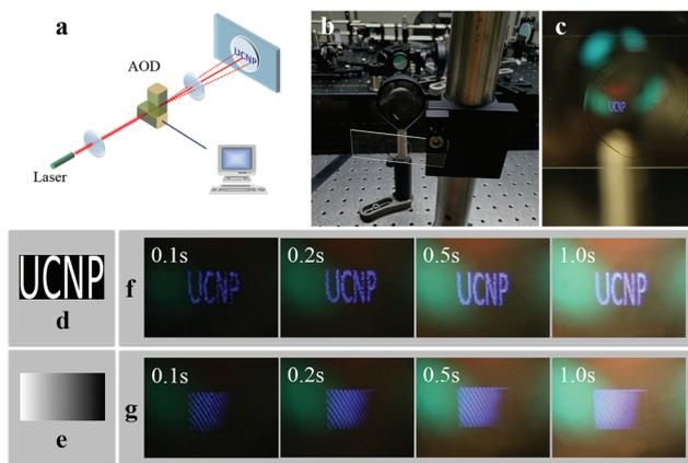
**Fig. 4** (a) Schematic of the computer-controlled scanning system that employs AOD and an optical lens to control light deflection and focus. (b) Photograph of the display system. (c) The letters “UCNP” displayed on the PVA film. (d) The “UCNP” pattern and (e) grayscale gradient pattern entered by a computer. (f) “UCNP” pattern photographs and (g) grayscale gradient photographs taken at different exposure times (0.1, 0.2, 0.5, and 1.0 s).
