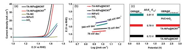
Fig. 5 (a) OER LSV curve for various catalysts at a scan rate of 5 mV s<sup>-1</sup> and a rotation speed of 1600 rpm after 95%-iR correction. (b) Tafel plots derived from the corresponding OER LSV curves. (c) The potential gap ( $\Delta E$ ) between the OER potential measured at a current density of 10 mA cm<sup>-2</sup> and the ORR half-wave potential.
