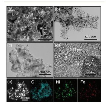
Fig. 1 (a) SEM image, (b and c) TEM images, (d) HRTEM image, and (e) dark-field image of TA-NiFe@NCNT. Element maps for C, Ni and Fe are also shown in (e)
