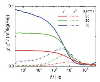
Fig. 6 ACS measurements of single core iron oxide nanoparticle samples T1 ( $d_c = 23$  nm), T2 ( $d_c = 30$  nm), and T3 ( $d_c = 36$  nm) synthesized at three different temperatures ( $\Delta T = 5$  K). The straight lines denote the real part, and the dotted lines the imaginary part of the complex dynamic susceptibility.
