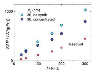
Fig. 9 Measured SAR values versus the frequency of single-core ironoxide nanoparticle system T2 (30 nm) as synthesized (cyan circles), and concentrated (blue circles) and of the MRI contrast agent Resovist®.
