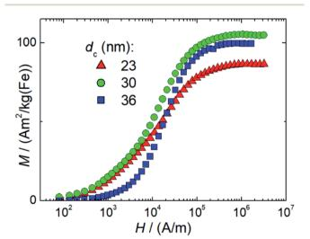
Fig. 4 Room temperature (T=295 K) DC magnetization curves of single-core iron oxide samples T1 ( $d_c = 23$  nm), T2 ( $d_c = 30$  nm), and T3 ( $d_c = 36$  nm) synthesized at three different temperatures ( $\Delta T = 5$  K).
