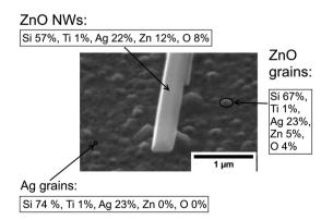
Fig. 8 SEM image of ZnO NWs grown on Ag (45  $^{\circ}$ C tilted) at a precursor concentration of 5 mM and growth time of 18 hours. EDX data (elemental percentage) have been shown at the points of ZnO NWs, ZnO grains, and Ag grains. The electron beam penetration depth is  $\sim$ 1  $\mu$ m; carbon and other contaminants have been ignored.
