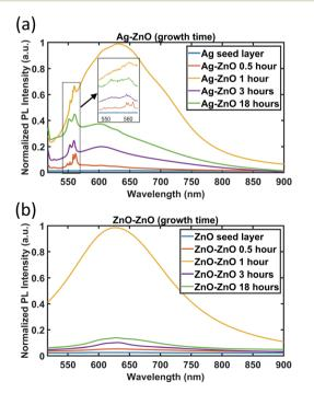
Fig. 9 PL spectra of ZnO NWs grown on (a) Ag and (b) ZnO seed layers as a function of growth time. For the Ag seed layer, the zoomed-in spectra between 550 and 560 nm are shown in the inset.
