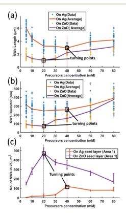
Fig. 6 ZnO NW growth as a function of different precursor concentrations (18 hours growth at a temperature of 90 °C): (a) length; (b) diameter; and (c) density.
