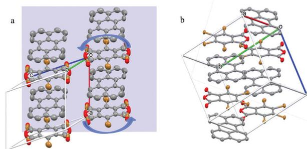
**Fig. 1** Unit cell of perylene–TBPA in (a) HTP at 290 K and (b) LTP at 150 K. Curved arrows in (a) are included to highlight the TBPA dynamic reorientation. In TBPA the coloured atoms indicate oxygen (red) and bromine (brown). In the HTP of (a) the bromine and oxygen atoms appear superimposed because of the dynamical reorientation. The background plane in (a) represents the crystal face used for optical reflectivity measurements. Unit cell parameters are reported in the ESI.†
