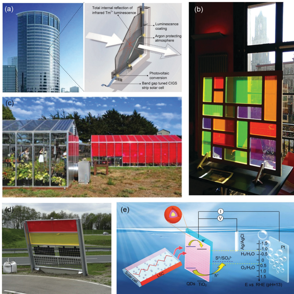
Fig. 15 (a) Schematic of a PV window consisting of a semi-transparent, colorless LSC. (b) Photograph of the Electric Mondrian prototype. (c) Photograph of the LSC greenhouse. (d) Photograph of the noise barrier prototype. (e) Schematic diagram of the CdSe/CdSSe/CdS QD sensitized photoanode coupled with an LSC based on CdSe/CdS QDs. (a) Reproduced with permission from ref. 28. Copyright 2015 Elsevier. (b) Reproduced with permission from ref. 149. Copyright 2017 Wiley-VCH. (c) Reproduced with permission from ref. 150. Copyright 2016 AIP publishing. (d) Reproduced with permission from ref. 151. Copyright 2017 Elsevier. (e) Reproduced with permission from ref. 153. Copyright 2019 The Royal Society of Chemistry.
