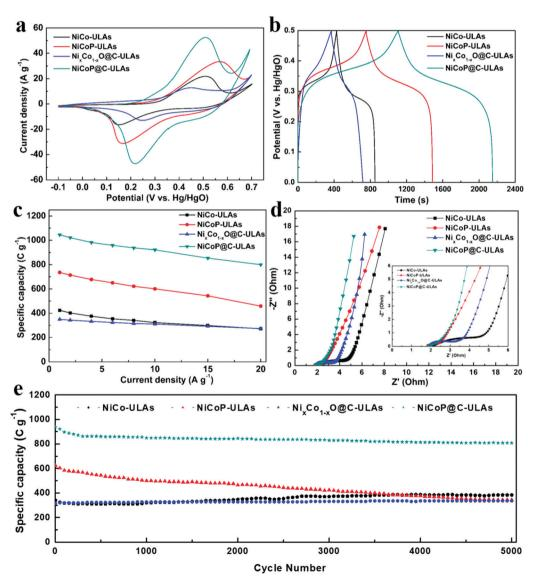
Fig. 8 Electrochemical performances of different electrodes. (a) CV curves at a scan rate of 10 mV s<sup>-1</sup>, (b) GCD curves at a current density of 1 A g<sup>-1</sup>, (c) specific capacity at different current densities. (d) Nyquist plots; the inset shows the high-frequency region. (e) Cycling performance at a constant current density of 8 A g<sup>-1</sup>.
