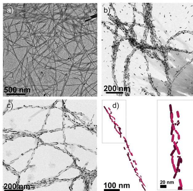
Fig. 10 (a) TEM image of  $\alpha$ -synuclein fibrils. (b and c) TEM images of  $\alpha$ -synuclein fibrils in the presence of AuNRs at 2 and 0.5 nM concentrations, respectively. (d) Cryo-TEM tomography reconstruction image showing a 3D chiral arrangement of the AuNRs. Reproduced with permission from ref. 121.
