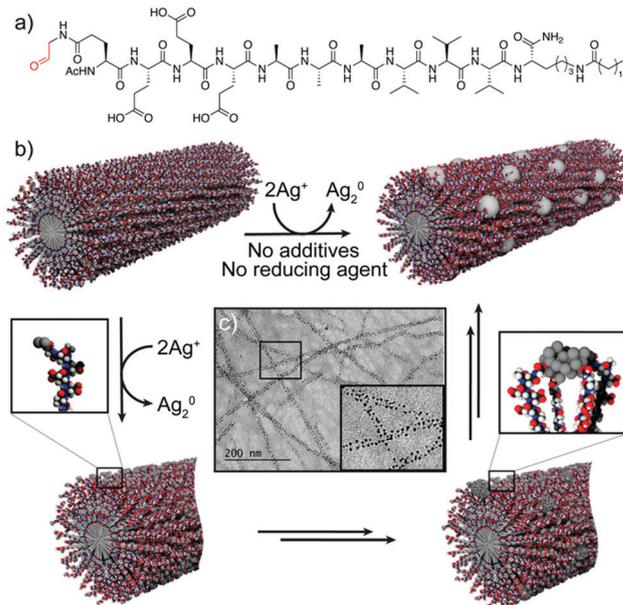
Fig. 4 (a) Chemical structure of the peptide–amphiphile. (b) Schematic representation of the proposed mechanism for the formation of peptide–AgNP hybrid nanofibres. (c) TEM image of the hybrid nanofibres. Adapted with permission from ref. 36.
