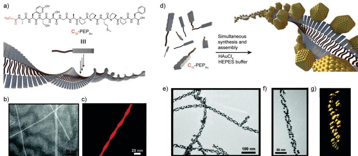
**Fig. 2** (a)  $C_{12}$ -PEP<sub>Au</sub> chemical structure and representation of its self-assembly into twisted-nanoribbons. (b) TEM and (c) AFM images of  $C_{12}$ -PEP<sub>Au</sub> nanoribbons. (d) Schematic representation of the AuNP double helices. (e and f) TEM images, and (g) electron tomography reconstruction of the peptide-AuNP superstructures. Adapted with permission from ref. 44. Copyright 2008 American Chemical Society.
