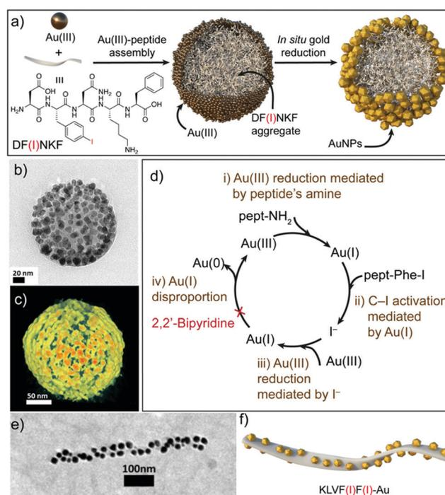
**Fig. 3** (a) Schematic representation of the formation of spherical DF(I)NKF-Au hybrid superstructures. (b) TEM image and (c) electron tomography reconstruction of DF(I)NKF-Au superstructures. (d) Representation of the gold reduction mechanism. (e) TEM image and (f) schematic representation of helical KLVF(I)F(I)-Au superstructures. Adapted with permission from ref. 37.
