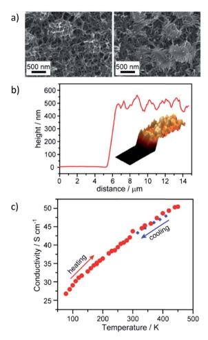
Fig. 10 a) SEM micrographs of Ni<sub>3</sub>(HITP)<sub>2</sub> films with 500 nm thickness measured via (b) AFM. (c) van der Pauw conductivity measurements at various temperatures show reversible increase in conductivity for 500 nm thick films on quartz. Adapted with permission. 168 Copyright 2014 American Chemical Society.
