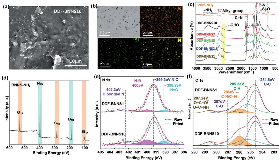
Fig. 1 (a) SEM and (b) TEM images and element mapping of DDF-BNNS10; (c) FTIR spectra of BNNS-NH<sub>2</sub> and DDF-BNNS samples with different BNNS-NH<sub>2</sub> content values; (d) the XPS spectrum of BNNS-NH<sub>2</sub>; and (e) N 1s core-level and (f) C 1s core-level spectra of DDF-BNNS1 and DDF-BNNS10.
