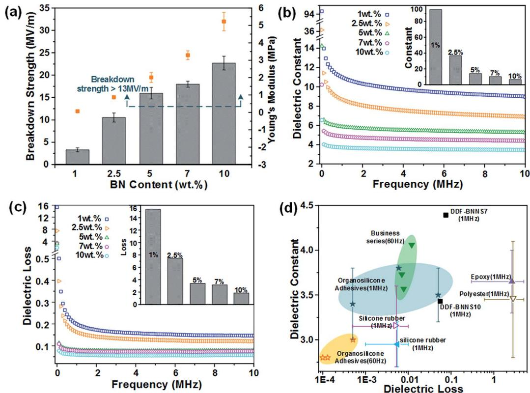
Fig. 4 (a) The breakdown strength of DDF-BNNS with different BNNS-NH<sub>2</sub> content. The frequency-dependent dielectric constant (b) and loss (c) of DDF-BNNS with different BNNS-NH<sub>2</sub> content; inset: dielectric constant (b) and loss (c) of DDF-BNNS with different BNNS-NH<sub>2</sub> content at 20 MHz. (d) A comparison of dielectric constant and loss values between different adhesives and insulating materials.
