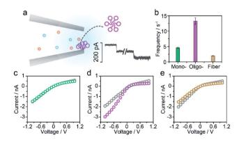
Fig. 3 A $\beta$ 1–42 oligomer sensing with glass nanopores. (a) The typical step like current fluctuations induced by the adsorption of A $\beta$ 1–42 oligomers onto the nanopore sidewall. (b) Frequencies of the pulse-like signals for the sensing of three types of A $\beta$ 1–42 peptides. I-V curves of the glass nanopore measured in the pure electrolyte before (gray) and after A $\beta$ 1–42 monomer (c), oligomer (d) and fibre (e) sensing, respectively.
