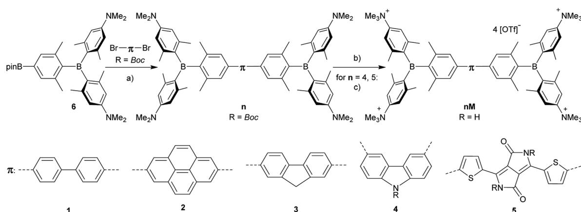
Scheme 3 Synthesis of compounds **1M–5M**. (a) [Pd<sub>2</sub>(dba)<sub>3</sub>] (dba = *trans,trans*-dibenzylideneacetone), 2-dicyclohexylphosphino-2',6'-dimethoxybiphenyl (SPhos), KOH, toluene, H<sub>2</sub>O, 85 °C; (b) MeOTf, CH<sub>2</sub>Cl<sub>2</sub>; (c) TfOH, MeOH.
