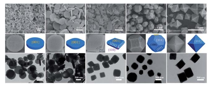
Fig. 2 SEM, enlarged SEM, TEM images and the corresponding 3D geometry models of as-synthesized NH<sub>2</sub>-MIL-125(Ti) obtained under different concentrations of CTAB: (a) 0, (b) 1 mM, (c) 2 mM, (d) 3 mM and (e) 4 mM.
