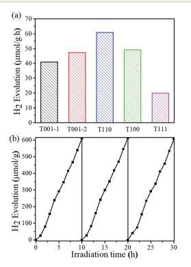
Fig. 4 (a) Photocatalytic hydrogen production using  $NH_2$ -MIL-125(Ti) with different morphologies. (b) Recycling tests using T110.
