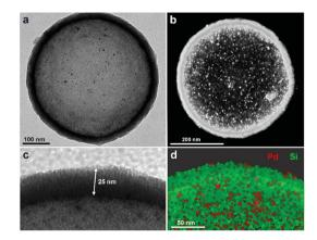
Fig. 2 Characterization of Pd-Cap1. (a) Representative TEM image (500 nm diameter); (b) STEM image; (c) zoom-in view showing the vertically oriented mesopores in the silica shell with a thickness of 25 nm; (d) XEDS mapping showing the elemental distribution of Pd and Si.
