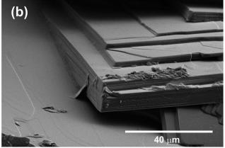
Fig. 2 CHLM crystals display a diverse surface topography. SEM images of CHLM crystals, which predominantly expose {001} surfaces – consistent with what has been reported in ref. 54. It is quite clear that these plates possess numerous topographical features.
