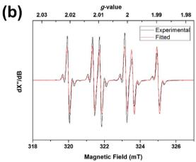
Fig. 7 Spin trapping of 2. (a) EPR monitoring of a toluene solution of 1 and PBN at -50 °C, under visible light irradiation (Xe lamp, 420–780 nm), and (b) fitting of the EPR spectrum of the same sample, recorded at -20 °C.
