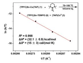
Fig. 9 Eyring plot of the reaction of 1 with TEMPO. Conditions: 1.6 mmol  $L^{-1}$  of 1, 16 mmol  $L^{-1}$  of TEMPO, toluene- $d_8$  (containing 15% v/v  $C_6D_6$ ), in the dark and under a  $N_2$  atmosphere.
