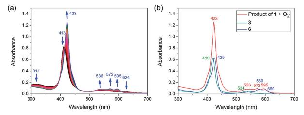
Fig. 3 (a) Photo-oxidation of 1 in aerated toluene over a period of 11 s monitored by stopped-flow UV-Vis absorption spectroscopy. (b) Comparison of the UV-Vis spectra of 3 and 6 with that of the product mixture.
