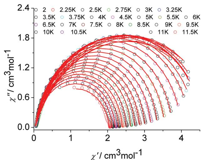
Fig. 5 Cole–Cole (Argand) plot for **1** obtained using the ac susceptibility data. The solid lines correspond to the best fit obtained with a generalized Debye model under a zero dc field.
