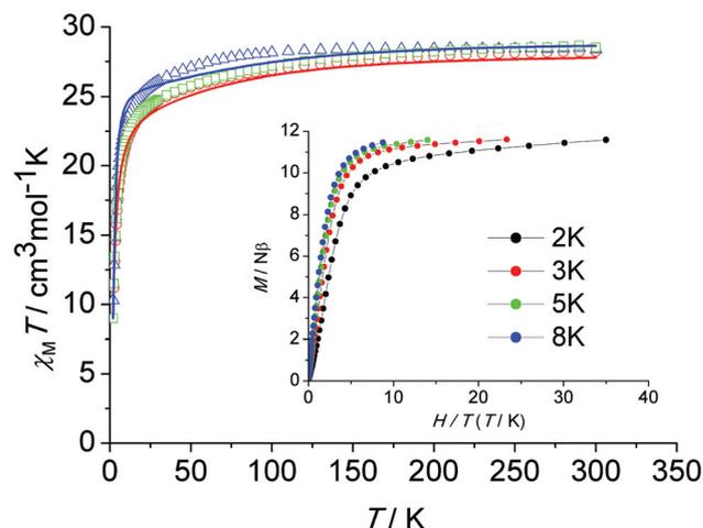
**Fig. 3** The  $\chi_M T$  data measured on powdered samples under a magnetic field  $H = 1000$  Oe for **1** (red circles; red line, best fit), **2** (blue triangles; blue line, best fit) and **de1** (green diamonds). Inset:  $M$  versus  $H/T$  plot for **1** at indicated temperatures.
